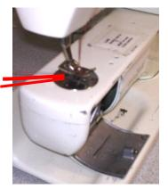
Tuck both threads under the presser foot and towards the back of the machine
