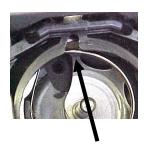
Note the finger on the bobbin case clicks into the slot at the top
