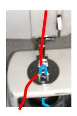
Hold the top thread & turn the wheel on the side of the machine forward to do one stitch – the needle will pick up the bottom thread & pull it up to the top of the machine
