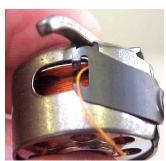
Slide the thread under the spring on the case
