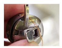
Open the latch on the case (keep the finger on the case pointing upwards)
