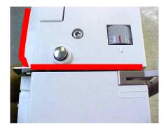
Lay the thread along the channel. Check the thread slots in between the hidden tension discs inside the channel
