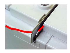
Place the thread under the hook at the back of the machine
