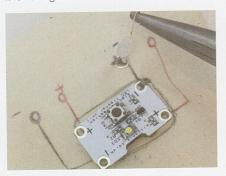
Oversew the positive side of the right hand side of the cell holder to the calico and use small running stitches to stitch along the red line to get to the positive point where the LED will sit and oversew the LED onto the fabric. The right hand side of the circuit is now complete and one LED is sewn into place. You can test the circuit by putting the battery into the cell holder and the LED will light up (remove after testing). Check the 'trouble shooting' section if it doesn't.
